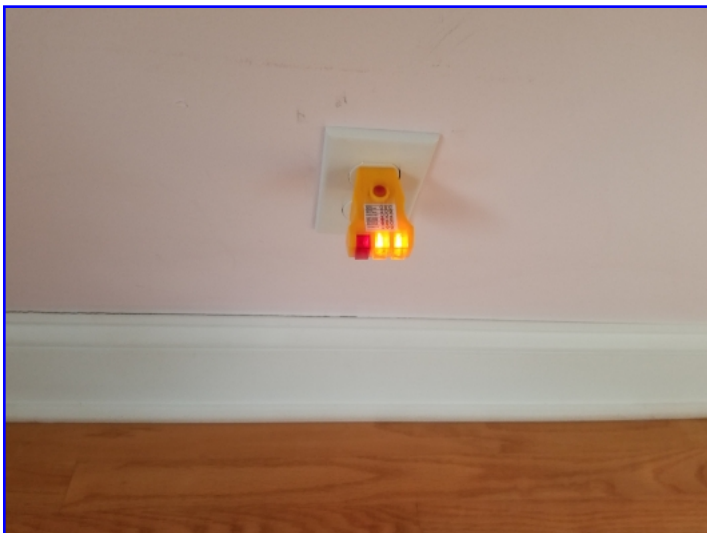
At the time of the inspection, the Inspector observed no deficiencies in the condition of electrical receptacles. In accordance with the Standards of Practice, the inspector tested a representative number of accessible outlets only.
